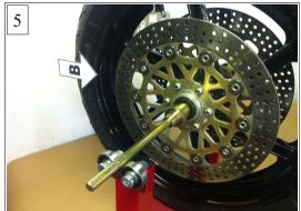
With the weight attached, set "point B" at the three or nine o'clock position and let go of the wheel. If the weight added goes back to the top and "point A" back to the bottom you need to add more weight (try adding another 10g) and repeat the procedure. If the weight (at point B) falls to the bottom you need to reduce the weight. You are aiming for a perfect balance.
