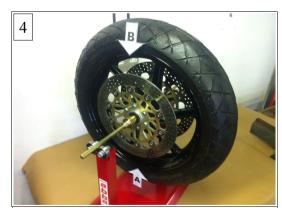
Now with the wheel in the same position mark the highest point of the wheel (12 o'clock). This is the lightest point or the counterbalance point (call it point B). Take one 10g adhesive weight (supplied) and place it flat inside the rim at "point B". Secure temporarily with sticky tape only as you may need to add or remove the weight.
