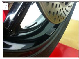
Remove the tape holding the weights (make sure this position is still marked). Clean the area using contact cleaner and attach the weight using the self adhesive backing (Tip- if cold warm the adhesive back before application) push weight on firmly. If the total added weight is more than 30g, divide the weight evenly and place either side of the rim. Finally perform a final check as in point 6.
