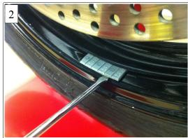
To balance a wheel you must first remove any existing wheel weights from the rim. The sticky back type can be difficult to remove cleanly, the simplest way is to insert a flat bladed screwdriver between the weight and sticky foam backing and gently flick off. Any residue left behind should be cleaned off with contact cleaner.
