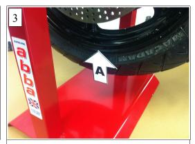
Slide the wheel balancer rod inside the wheel followed by the "abba staged adapter set" locate the correct stage of the adapter inside the wheel bearing of the wheel on both sides, this should be a nice snug fit. With the wheel now located on the balancer, gently spin the wheel with enough force for the wheel to complete three of four revolutions.
