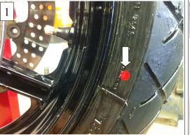
Time spent balancing a wheel can be reduced by ensuring a new tyre is correctly fitted to the rim. Most tyres include a balance mark denoting that the wheel's valve should be placed at this point when fitting the tyre. This will usually be a red dot or yellow circle. Check with the tyre manufacture if unsure.
