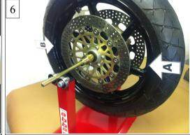
A perfect balance is achieved when the added weight point (point B) is positioned at three or nine o'clock and does not fall in either direction. Once you have got to this point, spin the wheel so slowly several times. It should each time stop in a different position and therefore have no favoured heavy point. If this is the case you have a very accurately balanced wheel.
