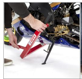
Next, with the bike leaning on its own prop/side stand fit the handle section of the stand to the left hand (near side) of the bike with the stand base in front of the prop stand, inserting the fitting into the hole or over the swing-arm pivot nut head.
