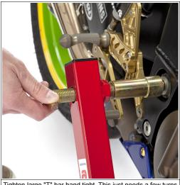
Tighten large "T" bar hand tight. This just needs a few turns to take the slack out of the stand (do not over tighten).
