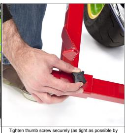
Tighten thumb screw securely (as tight as possible by hand).
