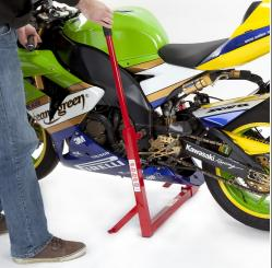
That's it! You should now have your bike sitting securely on the stand. Your bike can be left indefinitely in this position. To remove stand: Lower the stand by pulling handle towards the rear of the bike remembering to resist handle when stand passes pivot point. Then slowly lower to ground. Finally repeat the above steps in reverse order.
