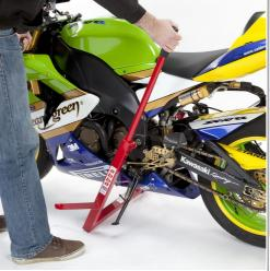
Stand the bike upright ensuring the handle bars are straight. Next, hold the handlebar of the bike with your left hand and pull out the extension lever to the top then lift bike with your right hand (pulling forwards).
