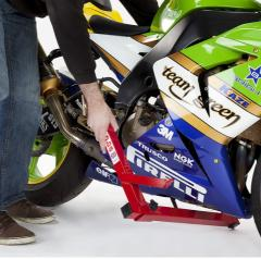
Walk around to the other side of the bike and slide the small section of the stand over the base of the handle section previously fitted, being careful not to push the handle section off. (Hold in place with left hand as per picture above).
