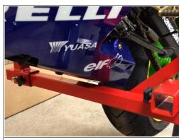
To lift the bike in the stoppie position (rear wheel high) simply pump the lift up with out any strap attached IMPORTANT: With the bike in both the wheelie position and the stoppie position you can lift until the base of the lift comes in contact with the underside of the bike as in the picture above. Do not go past this point or the lift will start to push against the bottom of the bike.
