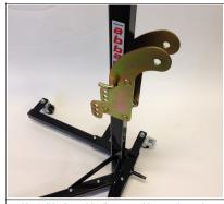
Next slide the gold roller assembly over the main upright of the lift and slide it down to the lower locking position. Line the holes up and slide through the locking pin so the roller assembly holds in place.
