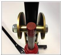
Pump the hydraulic pump up until the hole on top of the shaft is in line with the holes on the gold roller assembly. Fit the M16 nut and bolt using the 2 gold centralising spacers either side of the pump to keep the pump shaft central. Once again, when you have tightened the nut and bolt loosen it by around ½ a turn so there is some free play in the 2 centralising spacers.
