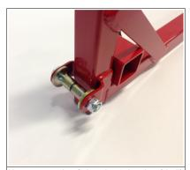
You are now ready to fit the red central section of the lift to the gold roller assembly of the sky lift. The two lower rollers have been pre set from the factory, do not adjust this bolt.
