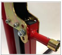
Slide the red section of the lift between the gold roller assembly plates and locate with the M14 nut & bott. You'll notice there is 3 different height options, we recommend you start with the middle position. You can later change this up or down depending on the height of your swing-arm pivot. (ensure the bottom roller guides on the red section sit correctly onto the main upright)
