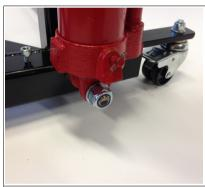
Fit the hydraulic pump by firstly locating it over the bottom pin and fitting the M16 nut and washer. Once you've tightened the nut, loosen it around ½ a turn to allow some free play in the pump on the bottom pin.
